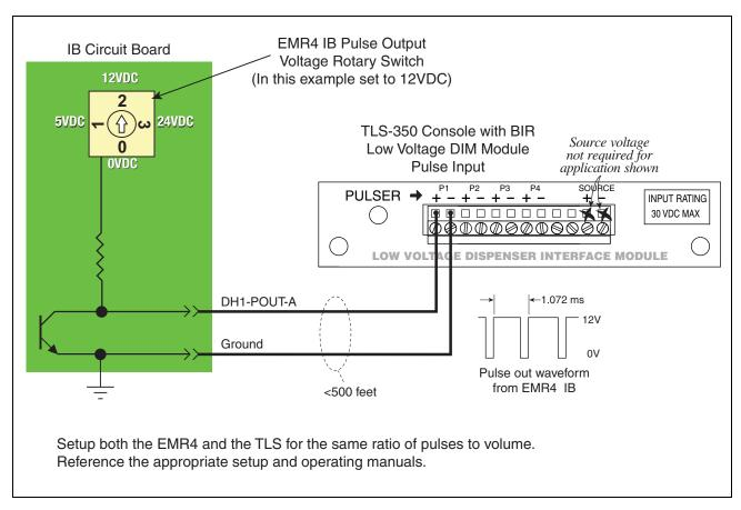
Figure 42. Wiring Pulse Output To A TLS-350 Console
