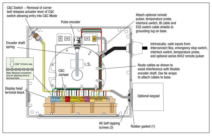
Figure 20. Display Head Cable Connections
