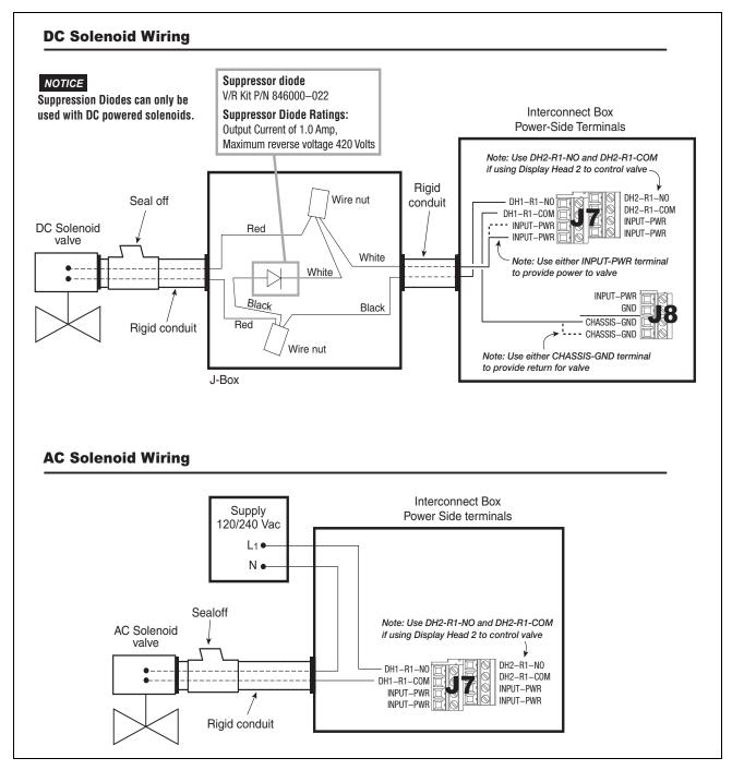
Figure 27. Example Wiring Connections For DC And AC Solenoid Valves
