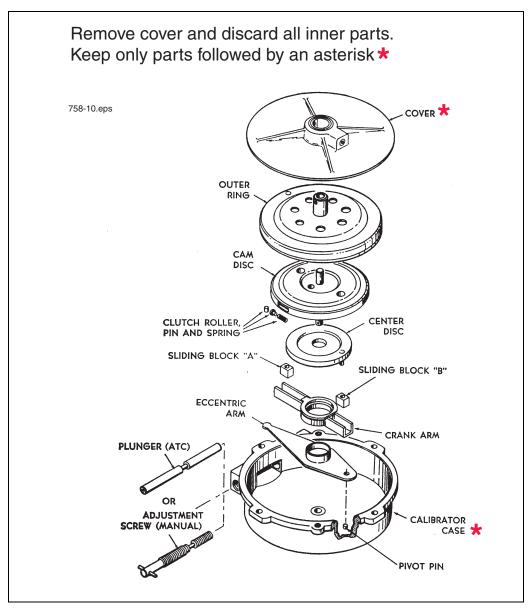
Figure 10. Disassembling The Smith Meter Calibrator
