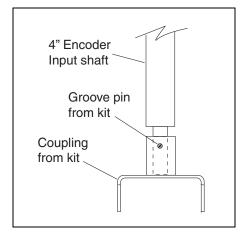
Figure 18. Attaching Coupling To Neptune Adapter Shaft
