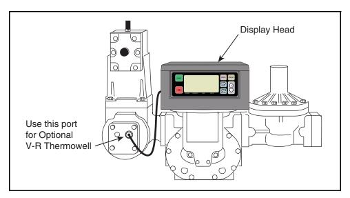
Figure 28. Example Thermowell Installation
