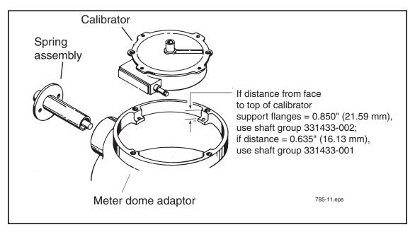
Figure 11. Calibrator, Spring Assembly, And Meter Dome Adapter
