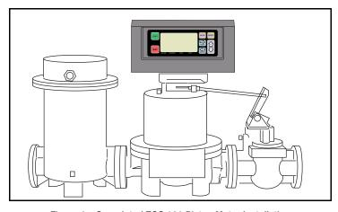
Figure 6. Completed TCS 682 Piston Meter Installation
