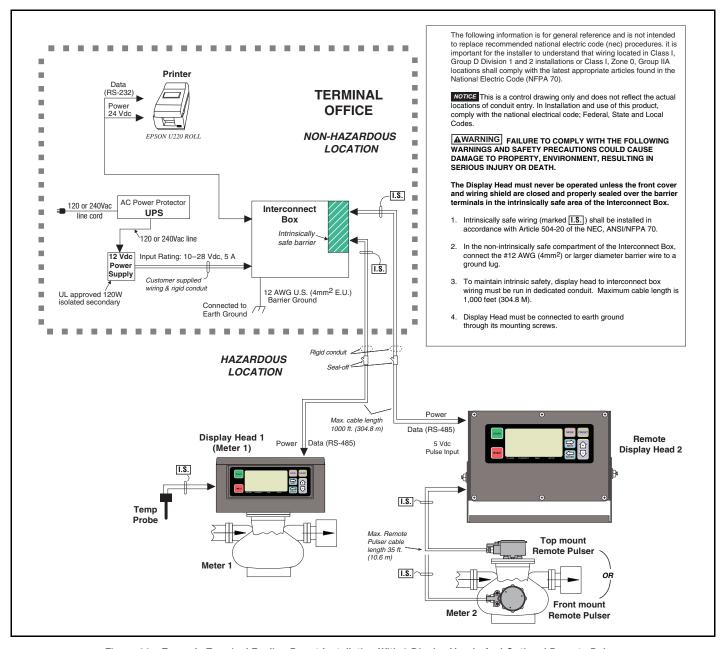
Figure 36. Example Terminal Fueling Depot Installation With 2 Display Heads And Optional Remote Pulser
