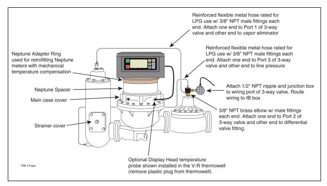
Figure 14. Example Of Temperature Probe Installation In Main Case Cover
