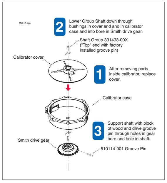
Figure 13. Reassembling The Smith Meter Calibrator
