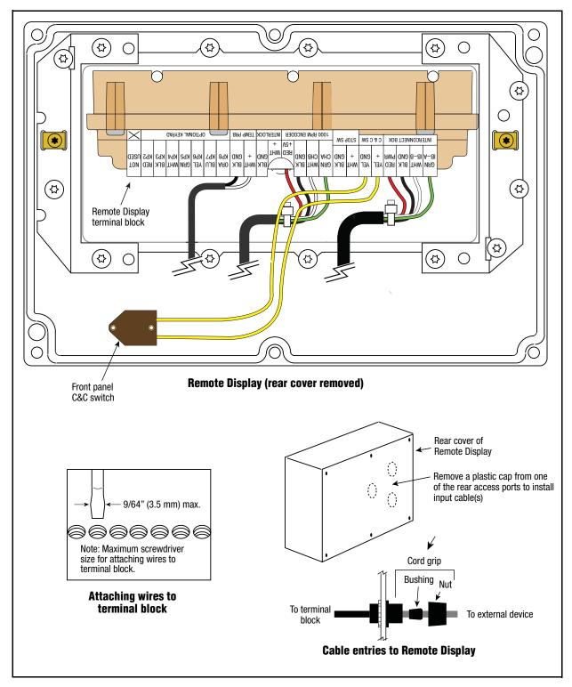
Figure 34. Remote Display Connections (Rear Cover Removed)
