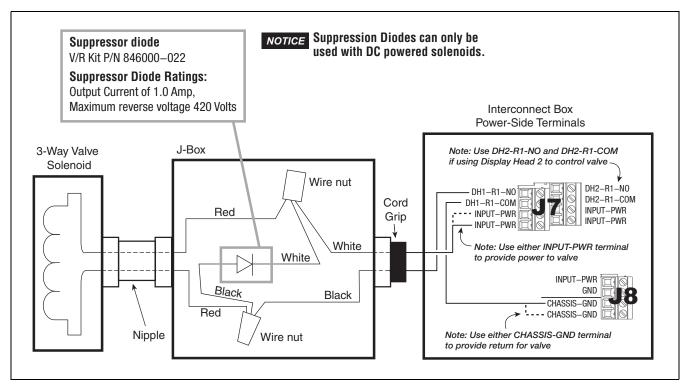
Figure 26. Connecting 3-Way Valve To The Interconnect Box
