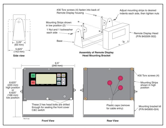
Figure 33. Remote Display Assembly
