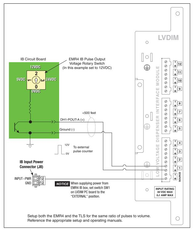
Figure 43. Wiring Pulse Output To A TLS-450/TLS4 Console
