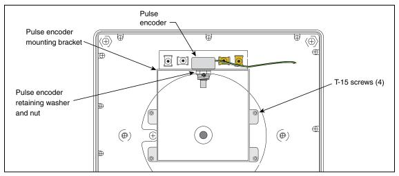
Figure B-1. Attach Encoder Mounting Bracket to Display Head Base
