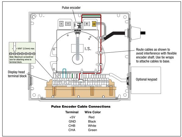
Figure B-5. Connecting Pulse Encoder Wiring To Display Assembly Terminal Block
