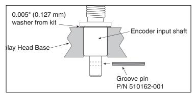
Figure B-4. Securing Encoder Input Shaft In EMR4 Base
