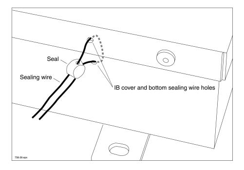
Figure 45. IB Sealing
