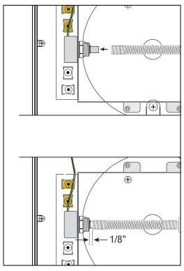
Figure 17. Pushing Encoder Spring Onto Pulse Encoder Shaft
