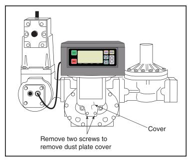
Figure 2. Remove Adjuster Dust Cover Plate
