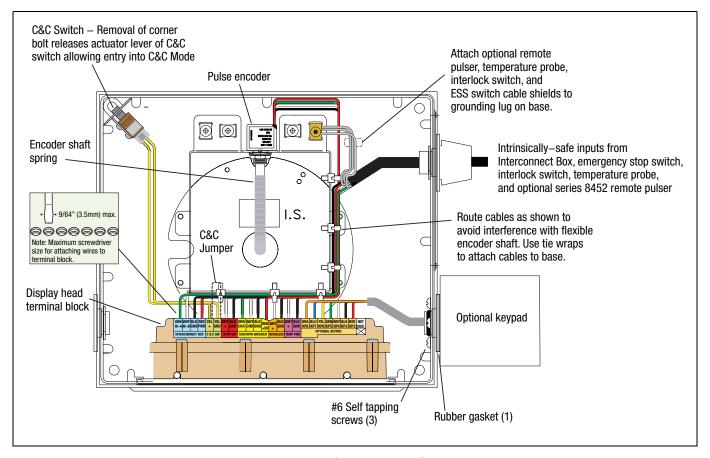
Figure 38. Display Head Cable Wiring And Switch Locations
