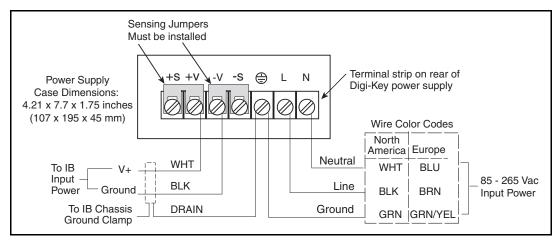
Figure 37. Digi-Key Power Supply Wiring Diagram
