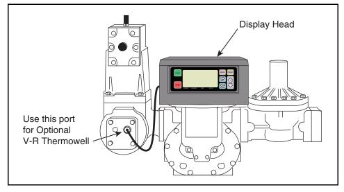
Figure 4. Example Of Temperature Probe Installation
