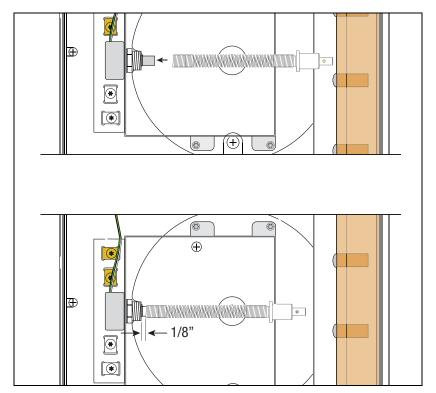
Figure C-3. Pushing Encoder Spring Onto Pulse Encoder Shaft
