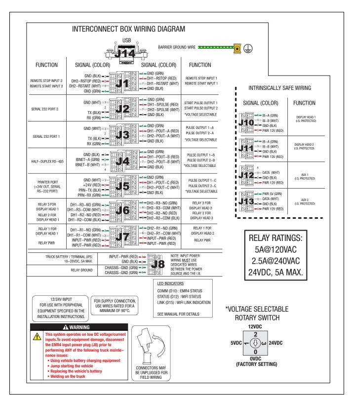
Figure 39. Terminal Interconnect Box Wiring
