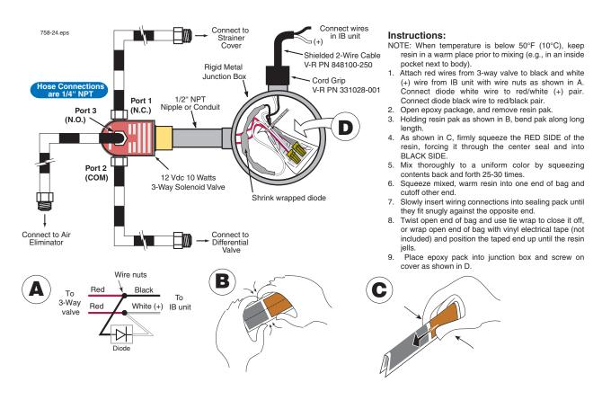
Figure 25. Connecting 3-Way Valve To L.C./TCS Meter - Truck LP Gas Installations
