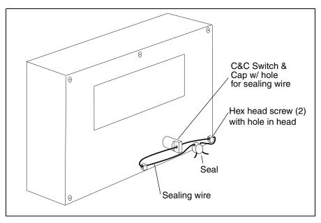
Figure 46. Remote Display Head Sealing
