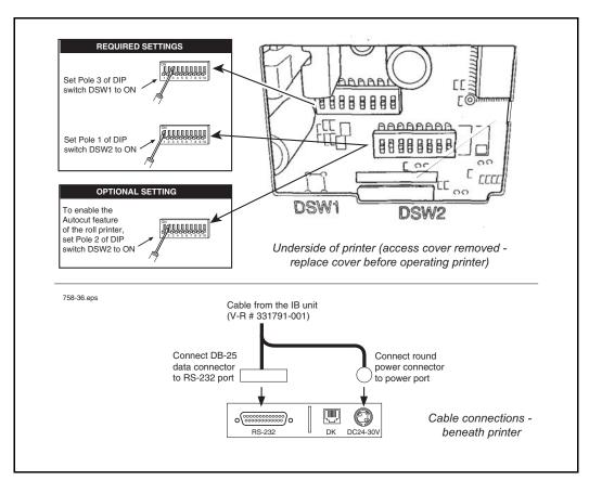
Figure 32. U-220A Roll Printer
