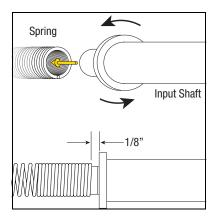
Figure 15. Screwing Input Shaft CCW Into Encoder Spring
