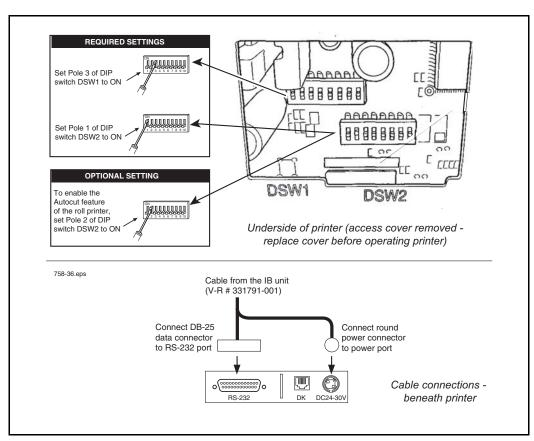
Figure 41. U-220A Roll Printer
