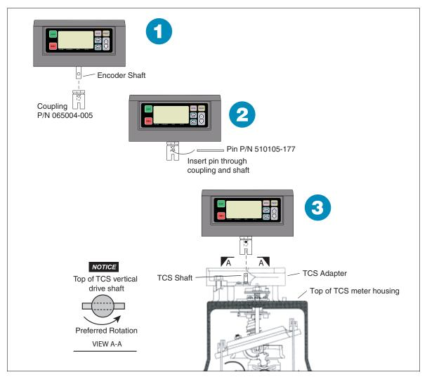
Figure 5. Display Head Mounted On TCS 682 Piston Meter
