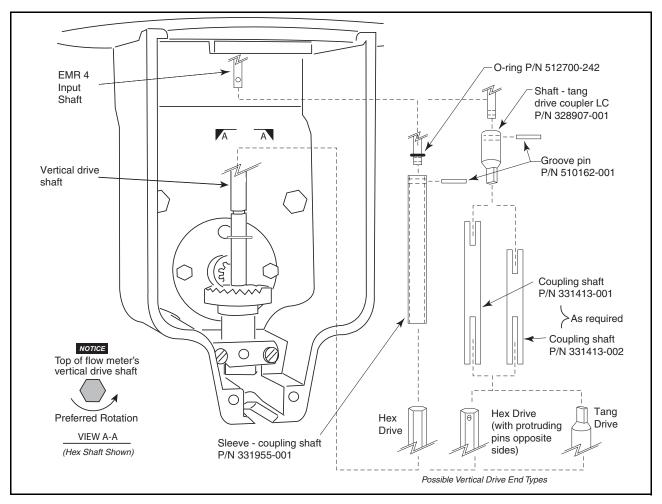
Figure 3. Installing Meter Encoder Adapter Coupling
