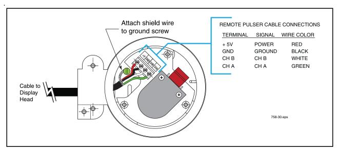
Figure 35. Wiring Connections In Remote Pulser (Top Cover Removed)
