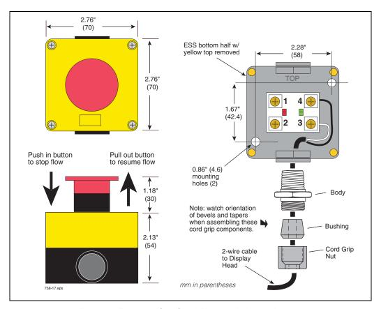
Figure 19. Emergency Stop Switch Mounting And Wiring Diagram
