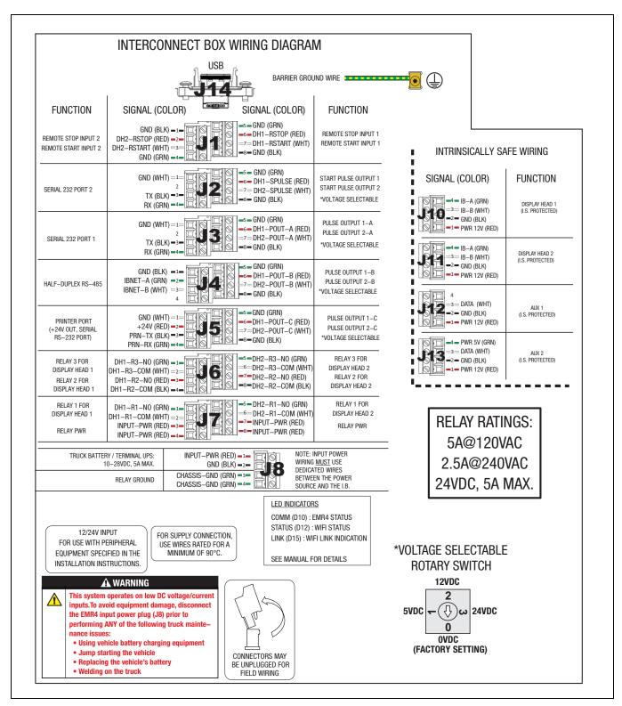
Figure 22. EMR4 Interconnect Box Wiring Connections
