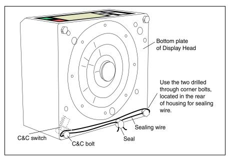
Figure 44. Display Head Sealing
